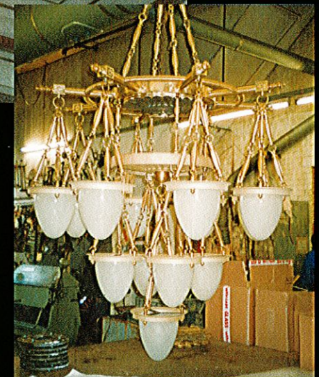
Inspection and testing of the pendant in our workshop before the final Antique Finish is applied
