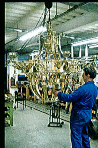
Final inspection of large multi-light pendant before being nickel plated
